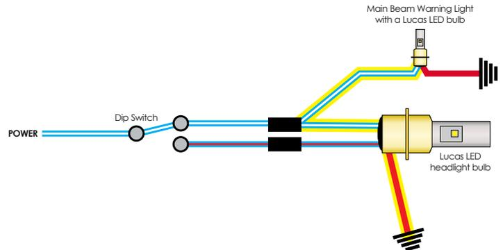
We have bench tested Lucas LED headlight bulbs using one of our positive ground Lucas LED warning light bulbs and the LED headlight bulb functions correctly. Dip beam lights one side of the LED and main beam illuminates both sides including the LED main beam warning light.
