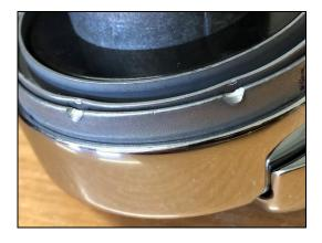
Use a small flat blade screwdriver, placed between the old cap seal and the retaining ring to carefully prise the ring up and out of the base of the fuel cap.
