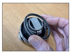
Once the old cap seal has been removed, the new seal can be fitted to the centre assembly. Refit the retaining ring ensuring that the indentations line up with those on the outer cap, this will help the ring to locate and seat correctly. Press the ring in with the flat blade screwdriver, again just a small amount at a time, moving around the circumference of the ring until it is fully seated.
