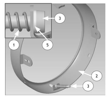
**7** Place the assembled Aero Visor on to the headlight and fasten the lower crosshead bolt into the light square nut until the bolt end passes through to the other side of the nut.
