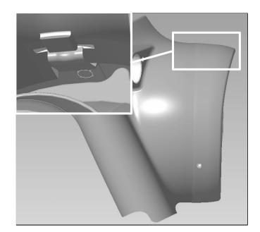
**11** Insert the 2x M5 Button Head Bolts (4) and torque to *6Nm*.
