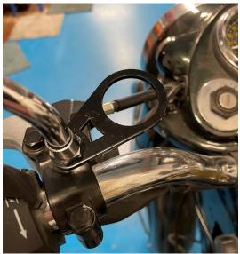
7. Fit the USB adaptor through this bracket and secure in place using the lock nut ring making sure the adaptor is positioned straight.
