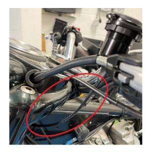
9. Connect the two-way block connector from the USB adaptor to the USB sub harness (The ones with Red and Black wires).
