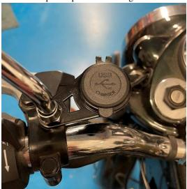
8. Route the braided wiring from USB adaptor in to the headlamp bowl. (Ensure there is enough excess wire allowing lock to lock steering without snagging or stretching).
