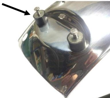
Plastic cup washers fit here and original 5mm screws used.
