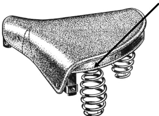
Bolt the two main springs to the rear of the underside of the saddle using 2 short M8 bolts into the outside of the three holes. Drop the other 2 M8 bolts and washers into the inside of the spring. This is easily done by bending the spring to open up the coils. Do not tighten any nuts until the saddle is fitted completely.
