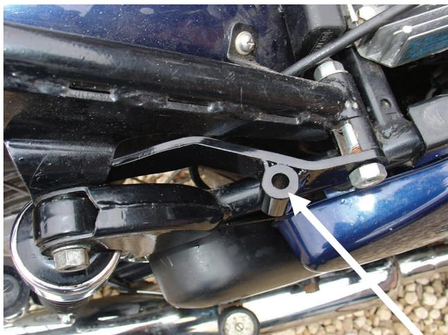
Attach the two Spring Support Brackets "B" to the inside of the rear suspension unit top pivot stud and the sub frame fixing stud (as picture) replacing the shock absorber bolts with the 3/8" bolts supplied
