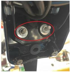
9. Remove the two extended nuts shown below, and remove the indicators from the holder.
