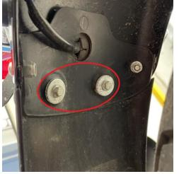
6. At the front of the rear mudguard, loosen the two screws circled below to allow the mudguard to drop.
