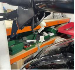
8. Remove the two screws shown below to separate the rear light holder assembly from the bike.
