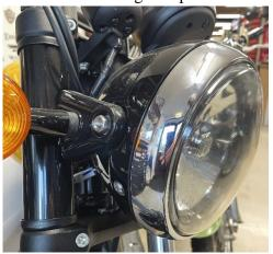
5 – Fit the headlight grille using the washers and screws supplied, and align the grille before tightening.
