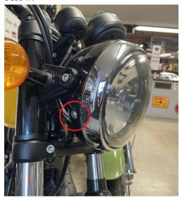
2 - Remove the main cap head screw from the headlight bowl.
