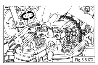
After setting correct gap, remove feeler strip, hold screw driver firmly such that the setting **DOES NOT** gets distrubed and gently lock the lock nut against rocker arm using special tool (a).
