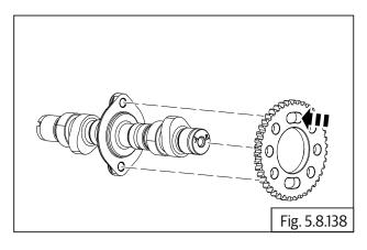
• Assemble cam chain **(a)** on sprocket and locate camshaft **(b)** into sprocket from the RH side.
