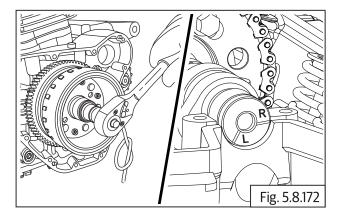
Ensure the angular edge of the special tool (a) is correctly located in the slot on the camshaft on RH side and the tool is resting correctly on the cylinder head.
