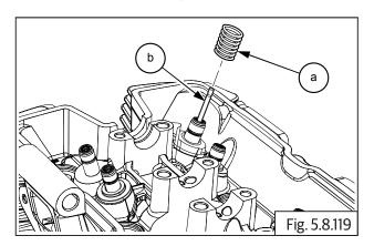
• Insert collar (a) above valve spring (b).
