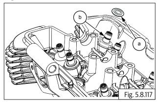
• Support the valve inside cylinder head and assemble valve spring (a) over valve stem (b) in the outer area of the cylinder head.
