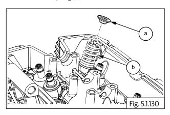
• Remove valve spring (a) from valve stem (b).
