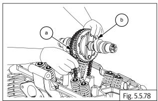
• Support timing chain suitably at the top to prevent it from dropping into the crankcase.
