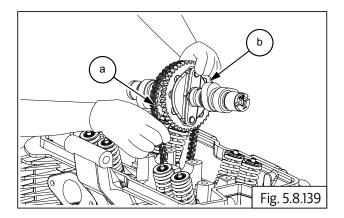
• Ensure reference mark "L" in the camshaft is aligned to the cylinder head on LH side.
