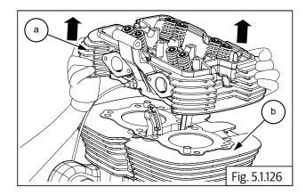
Remove the cylinder head gasket (a) from cylinder barrel (b).
