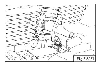
Assemble 2 Nos. Hex flange head bolt (M6) (a) on chain tensioner adjuster and tighten to specified torque.
