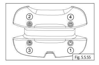
Gently remove rocker cover (a) from cylinder head (b).
