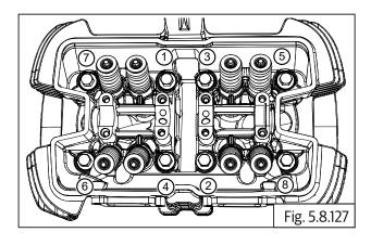
Finally tighten each of the cylinder head bolts using an angular torque wrench, to the specified angular torque value given below and in the same crisscross pattern detailed above.
