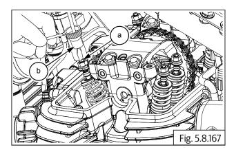
• Locate feeler strip (a) between adjuster screw and valve stem as per thickness mentioned below.
