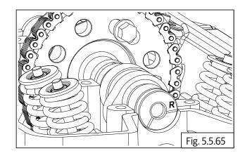
Loosen and remove 4 Nos. Hex head bolts (M10)
