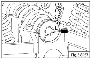
• Insert special tool **(a)** in crankcase RH to lock the crankshaft and prevent rotation.
