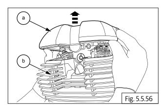
Remove rubber gasket (a) from cylinder head cover (b).
