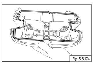
Locate cylinder head cover **(a)** on cylinder head with its narrow deep slot facing towards front of the engine.
