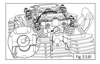
Loosen and remove 4 Nos. Hex flange head bolts
