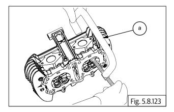
Repeat the above process to install the other seven valves, springs, collars and cotters on the cylinder head.
