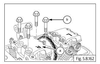
Tighten the bolts (a) to specified torque.
