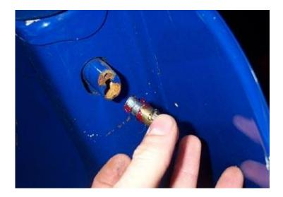
Clean the inside of the body area for the new lock. A blast of WD40 always works well. Make sure the little hole for the new rivet is clean and grease up the new lock and spring before inserting it into the frame hole.
