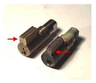
Be sure that you get a new lock that is the same as the one you are removing. There are two types of steering locks that look almost identical except for the flange on the top. The 4mm lock is shown on the right down below (after I drilled out the pins). On the left is a 6mm lock. Make sure you get the right one for your bike.
