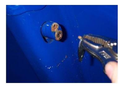
Using a pair of vice-grips, carefully grab the single rivet and turn and pull at the same time. Unless it is unusually stubborn it should come out of the body. Be careful to save the small washer that goes between the rivet head and the cover.
