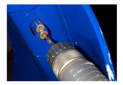
Next, chuck up the 3/8" bit and drill directly into the brass body of the existing lock. Take it slowly and only drill about 3/4" into the lock. What you are trying to do is destroy the small wafers that make the lock work so that it will turn with a flathead screwdriver.
