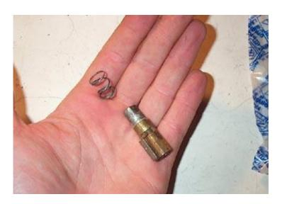
The new lock is just a single piece but the spring can be reused from the previous lock.
