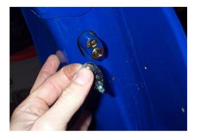
The rivet just need to be hammered into place. Fit the cap, small washer and rivet as shown above, and using a finish hammer (not a framing hammer with a waffled head) tap it far enough in that the cap won't rattle around when you are driving and the cover is not so tight it can't move.
