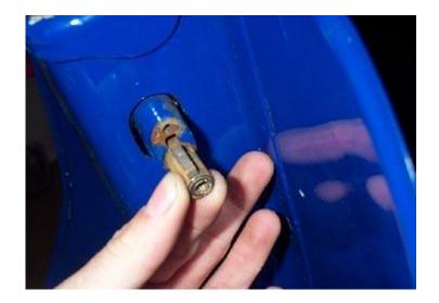
Once the wafers are destroyed you should be able to turn the lock about a 1/4 turn anti-clockwise. and then pull the entire lock body out of the frame as shown above. Save the small spring that should come out with it.
