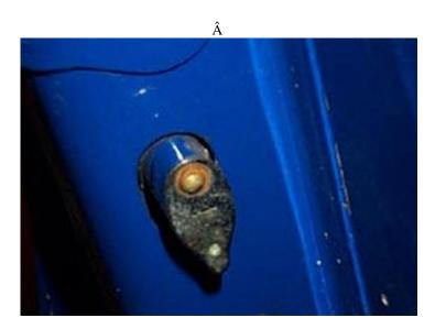
First, you need to remove the metal cover from the lock as it obscures part of the lock body from being pulled out.
