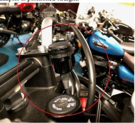
Route the braided wiring from USB adaptor through the cable guide and back alongside the frame. Ensure enough excess wire around the fork is left allowing lock to lock steering without snagging or stretching.
