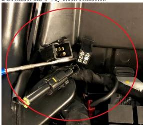
Plug the new block connectors from the USB sub harness in line with this, and tuck the connections back away to ensure they do not interfere when refitting the seat later on.
