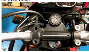
Place the USB bracket over the handlebar clamp and refit the bolts tightening to 20 NM. The USB bracket should have the large loop in front of the handlebars.
