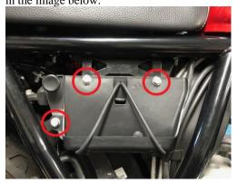
The cover should now be free to pull forward, and will just require the pull catch for the seat to be unclipped. This should simply push out of position as shown on the image below, to then allow the cover to be removed fully.
