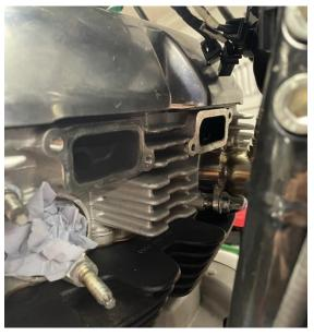
11. Fit the new blanking plate into place using the new gaskets and screws. Repeat for both sides.
