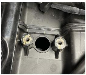
6. Using the plastic blanking plug from the kit, push this into position to seal the airbox.
