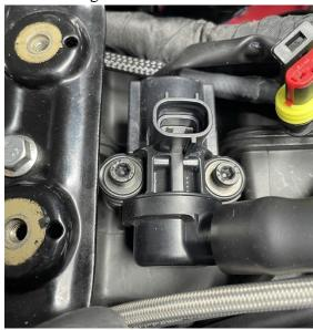
3. Fit the electrical connector supplied in the kit back into the bikes wiring loom.
