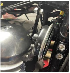
8. Remove all four screws holding the two covers.
