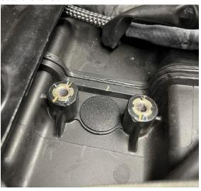
7. The reed valves are located at the front of the cylinder head to give better access to this area, it is best to remove the horns. In our photos we show this with the exhaust pipe removed, this is only to make the photos clearer and not needed in normal practice.
