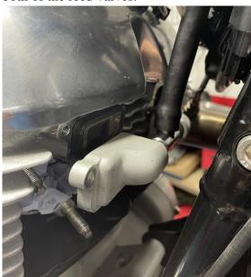
10. Remove the two covers, link pipes, solenoid, and associated parts as one unit from the bike, these will not be reused.
