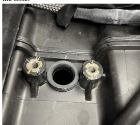
5. Remove the rubber grommet from the air box.
