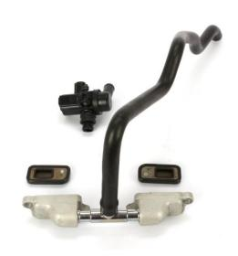
2. Identify the solenoid located on the top side of the airbox, disconnect the electrical connector, and unscrew the two retaining screws.
