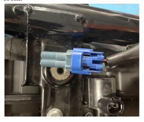
4. The solenoid assembly can now be pulled away from the airbox to expose the hole.
