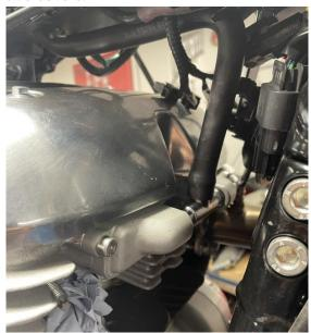
9. Pull the covers forward and remove both of the reed valves.
