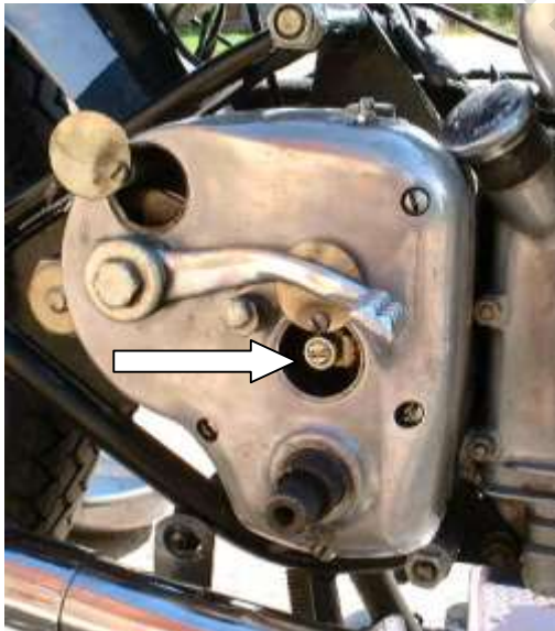
CLUTCH ADJUSTMENT ON GEARBOX
