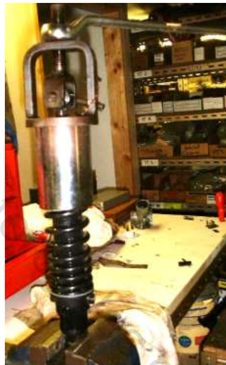
REAR SPRING BOX REMOVAL
