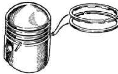
CORRECT RELATIVE POSITIONS OF DUAL SCRAPER RINGS (LATER MODELS)
