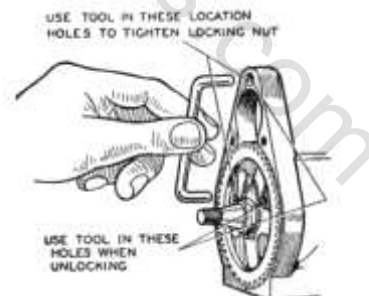
USE OF JIG FOR MAGNETO SLIPPING CLUTCH Fig. 46
