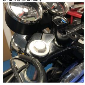
4. Beneath this is a flat solid washer, lift this out (sometimes it sticks to the threaded cap). Both this flat solid washer and the original fork cap are no longer needed and can be set aside.
