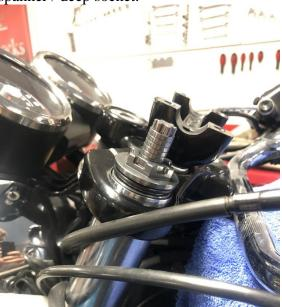
6. Repeat this for both sides, and set the pre load to the same height on either side. The rings can be used as a reference point to match the heights. Refit the handlebars in place (Interceptor only) and refit the bar clamps.
