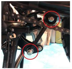
The new drop links come supplied with the bearings and seals already fitted, the only component you will need to transfer from the original assembly is the inner sleeve. This sleeve is just
