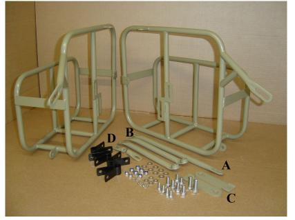
Fit lower bracket B, which you affixed to the frame previously, to the front Q Clip using M8 20mm Bolt, Nut and Washer
