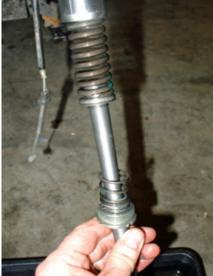
Fit the oil control collar on to the fork spring stud, with taper facing upwards. Again, a little grease will help to hold it in place on the spring stud.
