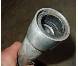
For the next step, we strongly recommend the use of the special tool, part ST25114 'Fork oil seal removal sleeve'. This tool slips over the top of the alloy fork end and prevents excess leverage cracking the alloy whilst removing the seals. With this sleeve in place, use an old tyre lever or strong screwdriver to lever out the first fork seal, then the nylon spacer and finally the second
