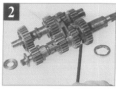
may not) be a similar flat-faced shim fitted to the bearing's offside, i.e. within the housing. And on the left is the thicker hardened thrust washer of smaller diameter which MUST be fitted between the kick starter pinion and kick starter shaft.
