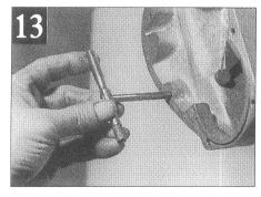
casting's fixing holes which ideally should be run through with the right size tap (picture 13).
