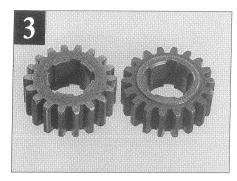
making up first gear. Note one of them is 'stepped'. Although this duo should be quite tightly fitted to their respective shafts they often seem to be transposed and/or fitted back to front.
