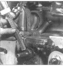
made of mild steel and can be easily damaged. It is very important, therefore to use a screwdriver that is a good fit into the screw's slot, so good in fact that there is no risk at all of it slipping and damaging the head. Do that and the screw will need to be chiselled off and the remainder drilled out.
