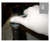
To reassemble the unit, grip the bottom casting in a vice and screw the main spring tightly into the bottom scroll (counter clockwise). Slide the lower cover over the spring, slide the upper cover over the lower cover. Insert the inner main tube in the spring. With a suitable bar through the top bush eye, screw the spring tightly into the upper scroll (counter clockwise). Screw the upper and lower covers in position.
