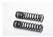
Another option is to fit dual rate springs, available for certain models. These springs give a softer ride and improved road holding. New springs ought to be fitted when the springs have 'set' by more than  $^{1}/_{4}$  inch. Any of these jobs will require dismantling the shock absorber units.
