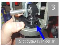
One type of Armstrong style unit uses two springs. These units are a little more complicated than the standard items but the method for dismantling them is the same — once the split collets have been removed the entire unit is easily dismantled.
