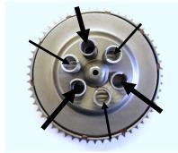
clutch plates. If a combination of heavy and light springs is used, fit the springs alternately: one light, one heavy spring (as in the picture on the right).
