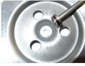
With the clutch dismantled, examine the components. Check that the tangs on the
