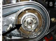
Before replacing the rotor, slide the rotor spacer onto the shaft and replace the rotor woodruff key followed by the rotor. Locate the rotor lock-washer and nut and tighten to 40lb/ft. (photo 9). Position the three stator spacers on their studs and replace the stator, the lock-washers and nuts before tightening these, ensure you have an equal air gap between the rotor and stator otherwise serious damage may occur. An
