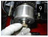
alternator clearance gauge makes this task simple—Hitchcock's part number 98240 or you can use a suitable piece of cut up plastic from an old coke bottle which can be wrapped round the rotor. Once in place the 3 stator nuts can be tightened, the plastic removed and a final check to ensure there is still an air gap.
