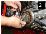
Because the primary drive uses an 'endless' chain, both the engine and clutch sprockets must be withdrawn together with the chain, as one complete assembly. To facilitate this it is necessary to remove the alternator stator and rotor. Remove the stator by undoing the three holding nuts (photo 2)
