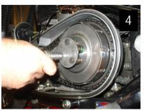
Slacken and remove the three clutch spring pins. Lift away the springs, the outer clutch plate and clutch pad, ensuring that any ball bearing, if fitted, does not drop out of the end of the gearbox mainshaft (photo 4).
