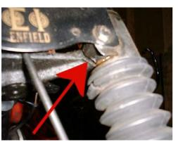
Unscrew the two shrouded nuts holding each of the two wheel spindle clamps. Remove the clamps, followed by the
