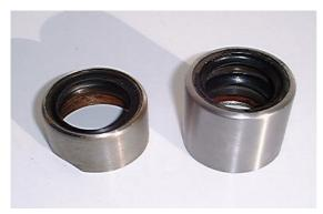
Early models had a single oil seal fitted in each holder. Later models have 2 separate seals fitted in a deeper holder. The later type, are far superior and can be fitted without problems to the early models. Most spares dealers will supply the later type as a matter of course.
