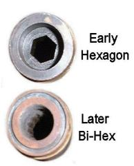
pressure exerted by the spanner normally clamps the seal holder on to the alloy thread even harder. If you are lucky, a bit of old inner tube and a strong grip will unscrew the seal holders, but normally a chain fitter wrench (as used on car oil filters) will be needed. This, no doubt will damage the surface area of the seal holder, but as these are throw away items, it will not matter.
