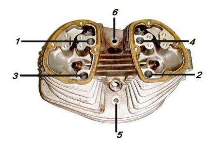
Refit the valve stem caps, pushrods, rockers and bearings tightening the 8 nuts to the correct torque, 9 ft-lbs. (If you have the alloy Samrat rockers the manufactures recommended torque is 5 ft-lbs).
