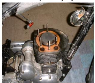
worn or the common problem of wet sumping is present. Hard shiny carbon would indicate a rich fuel mixture). Check all parts for signs of wear or damage and replace if necessary. Ensure that the valves are seating correctly and lap in with a fine grinding paste if required. Wash all parts in paraffin and reassemble the valves and collars, giving the top of the valves a light tap to ensure that the split collars have seated correctly.
