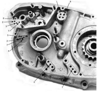
lodging place for small pieces of debris, usually hard jointing compound, and the only sure way of cleaning it out is to use a drill. If the hole is only half blocked, oil and air will still be able to pass through giving a false impression. Using a 4" long
