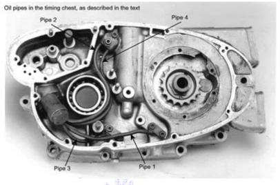
for about 1", to resume the horizontal line to connect with pipe no.3. Since a drill cannot go round corners, the vertical section is drilled from outside the case and the end of the drilling plugged with a short <sup>1</sup>/<sub>4</sub> BSF screw or bolt.
