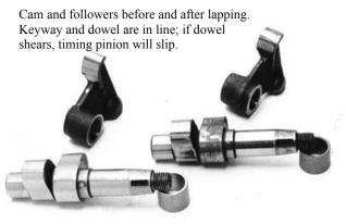
moment?), and it is therefore better to rectify the trouble straight away. Careful work with a drill is required to remove the sheared part, and a new dowel can be made from a piece of 10-gauge spoke.
