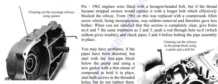
Repeat the procedure with the two-pipe junction at the top and then tighten all four screws home. The two single pipes are more flexible and can be manoeuvred into place and tightened too.
