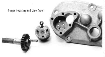
the 1957/8 models as these used the bigger feed plunger as standard. Inspect the peg closely for cracks as very occasionally they can break off, with disastrous results.
