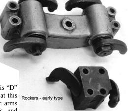
check the position of the inner arms; they should be level. If one is higher than the other, either the metal has worn off the end in contact with the valve or the D-hole has moved round on the spindle, in which case one or both will have to be renewed. The rocker bearing and rocker cover stud are 26TPI and stripped threads in the alloy head are not uncommon -
