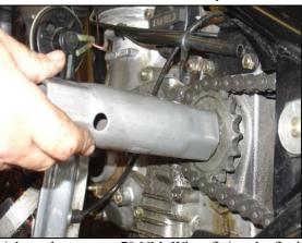
forgetting to bend the tab once the sprocket nut is tightened to approx 70 NM. When fitting the final drive chain ensure the split link is fitted with the closed end facing the direction of travel. Check the oil seal behind the clutch (111888) and if there are signs of damage or wear replace along with its gasket (144624). Be careful when sliding the seal over the shaft that you do not cause damage.
