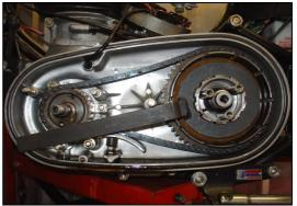
reassembling the clutch. To remove the clutch centre retaining nut, lock the clutch with the clutch holding tool (ST25104) and undo the large nut. Using the clutch puller tool (ST25099) remove the clutch centre from its splined shaft, the sprocket comes away with the centre.
