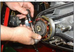
cables. Be careful not to lose the three small spacers, one on each of the studs that support the stator.
