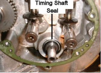
oil circulation. To prevent future problems always thoroughly clean all the oilways with a piece of stiff wire, when overhauling the engine and resist all attempts to cure oil leaks with excessive jointing compound. Put about half a cup of oil in the crankcases before replacing the barrel and piston. Pour a similar amount in the timing chest via the tappet inspection cover, this will help oil circulate around the engine faster on the initial start up.
