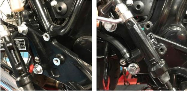
3. Attach the original foot peg hanger to the threaded holes in the adjustment plate using the original flanged M8 bolts. Reattach the brake master cylinder and guard to the foot peg hanger with the M6 cap head screws.
