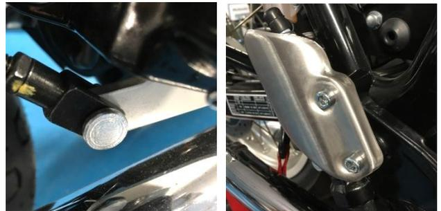
1. Remove split pin and fulcrum pin from brake lever/brake cylinder joint. Loosen M6 cap head screws and remove brake cylinder guard.
