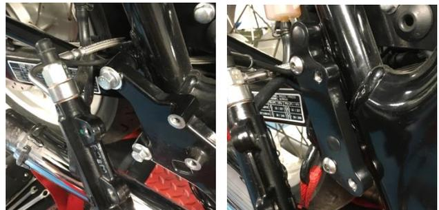
2. Carefully move the brake master cylinder to access the foot peg hanger. Remove the M8 flanged bolts and remove the foot peg hanger. Synchronise the position of the mounting holes on the adjustment plate with the gear change side. Attach the adjustment plate to the frame using the M8 x 30mm button head screws, (depending on the position you
