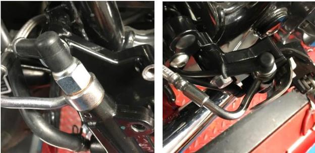
4. Depending on how the brake pipes were fitted at the factory you may have to carefully loosen the brake pipe nut to allow you to turn the brake pipe to clear the bracket. If this is the case there are spacers and longer cap head screws in the kit so you can still fit the guard.
