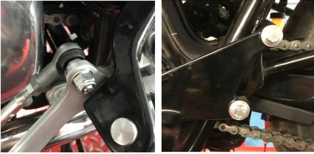
1. Undo the gear change linkage (10mm nut) and remove the connection from foot gear change lever. Undo foot peg hanger 12mm bolts and remove foot peg hanger.
