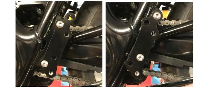
2. There are four recommended positions on the adjustment plate by using the two different untapped mounting holes and turning the plate over. (There are other positions but care must be taken if using these that the brake and gear lever have full travel and that any associated fittings/pipes are not stressed and cannot be trapped).
