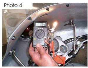
Regular attention to the battery will prevent many problems and avoid poor lights or starting difficulties. Always top up with distilled water and keep the connections clean and tight.
