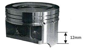
To calculate the final cylinder bore size measure 90° to the gudgeon pin, 12mm from the base of the piston skirt as indicated on the piston and add the recommended bore clearance. A 'plateau' microinch (CLA) would ensure best piston and ring running clearance.
