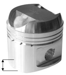
To calculate the final cylinder bore size measure 90° to the gudgeon pin, 15mm from the base of the piston skirt as indicated on the piston and add the recommended bore clearance. A 'plateau' hones finish of 25-30 microinch (CLA) would ensure best piston and ring running clearance.
