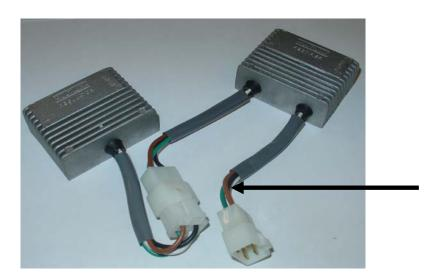
These two units can be disconnected at the female block connecter shown above by the arrow. They can then be discarded. The male block connecter left in the harness can be cut off and insulated and the Powerbox is then connected to these leads.
