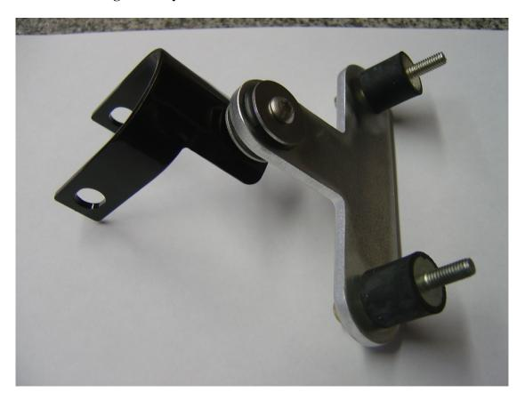
Screw the 2 bobbins to the rear underside of the alloy tank (using some thread lock may help any future dismantling of the support bracket)
