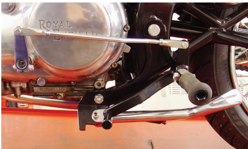
Left Side Pedal Assembly with Sidestand Fitted
