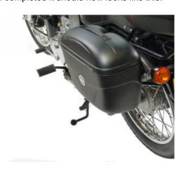
... then push the upper part of the pannier box towards the top locking latch. It should click into position.
