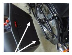
Drop the pannier box down onto the lower spacers first . . .
