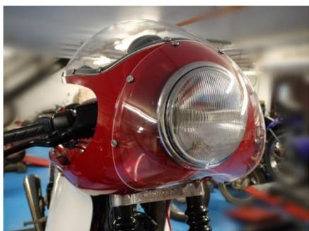
37. Locate and secure screen and headlamp cone
