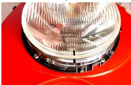
2. From the headlamp assembly fitted to the fairing remove outer rim from headlamp assembly – secured by a screw at bottom of rim
