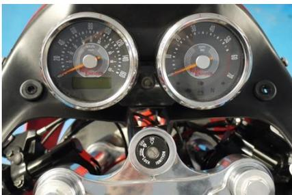
28. Fit instrument assembly into the instrument panel and secure with 4 x dome nuts and 4 x washers – note: lightly greasing the fixing studs will help fitting
