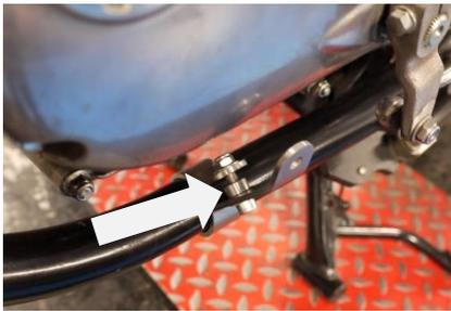
19. Locate and loosely assemble left-hand lower mounting clamp [F1]– note: use of spacers arrowed in photo
