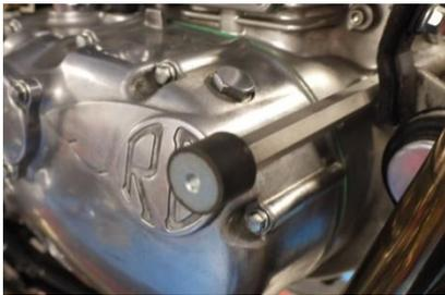
18. Locate and secure rubber bobbin to each hex mounting studs
