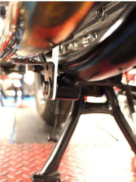
21. Locate and loosely assemble right-hand bottom bracket [F2] [highlighted white in photo] using original screw and washer
