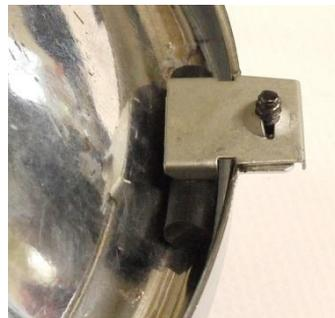
7. Locate 3 x rubber strips – secure with 3 x captive nuts and 3 x self-tapping screws
