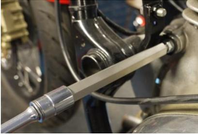
16. Remove the engine mounting screw securing the two horns and replace with the stud and nuts supplied [G] – leave equal length of thread each side of engine
