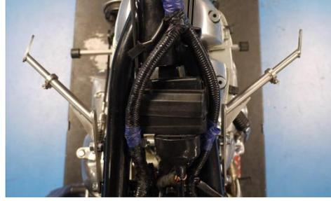
23. Locate and fully secure rear top mounting brackets with 4 x headsteady screws – these brackets are handed and marked 'L' and 'R'
