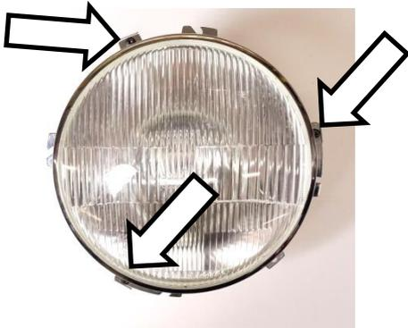
5. Remove x 3 crosshead screw and clips – arrowed in photo
