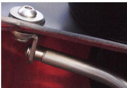
15. Locate and loosely secure one 'L' shaped end bracket [C] at each end of the front bracket. These screws to be fitted with low-grade thread-lock compound.
