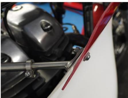
31. Position right-hand fairing lower section and secure with 5 x button head screws – see top left photo on page 5 – first secure fixing into the rubber bobbin and tighten with care
