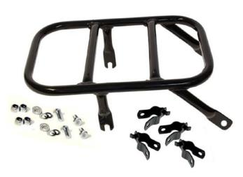
Working on one side at a time, attach one Q Clip to the rear of the mudguard rail as in photo below left (Due to variances in mudguards, it may be necessary to apply a bit of thumb pressure to the mudguard or slacken the mudguard to stay bolts to allow the clip to pass between the mudguard and stay). Using the supplied bolt, nut and washers attach the slotted stay of the carrier to the front of the Q clip as shown and lightly tighten.
