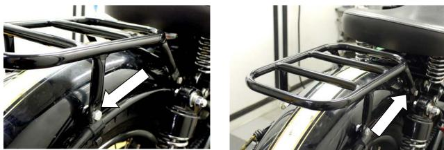
Attach one Q Clip to the front of the mudguard rail as in photo above right. Locate the forward stay of the carrier against the front of the Q clip and pass a bolt and washer through the assembly from behind. Finally secure that bolt with M8 Nut and Washer.
