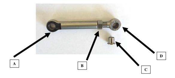
The head-steady assembly comprises four parts – see photo: A, B, C, and D. All four components can be orientated in different ways to provide approximately 20 adjustment positions to take account of variations in fittings.
