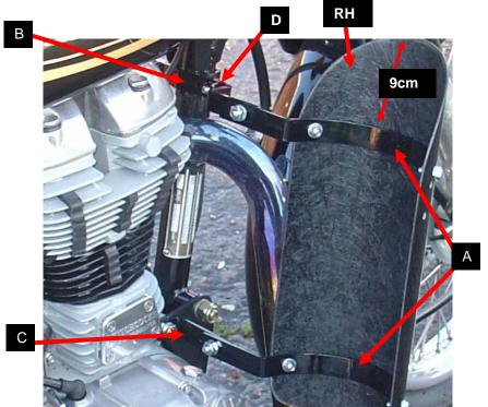
The Leg shields are not pre-drilled, as the positioning may vary depending on what indicators are fitted. Therefore, fix the mounting brackets in place first, using the 8mm screws and nuts provided.
