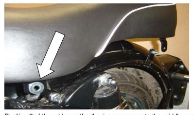
Once you are satisfied with the final fit remove the seat and tighten all brackets on the underside of the seat.
