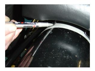
Fig 4 shows the bracket placed to the marks made previously and the slot positions that are then marked prior to drilling.
