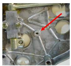
6. The gearbox cover central mounting hole needs to be enlarged, to enable the fine threaded Allen screw to pass through (arrowed). You will require a 7mm drill bit for this.
