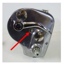
8. Once the cover is back on, the fine thread Allen head screw from the stiffener assembly kit passes through the original eccentric spacer for the neutral selector adjuster. Re-adjust as required.
