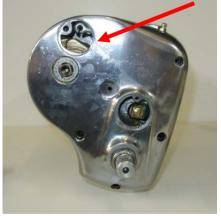
2. Disengage clutch cable (arrowed). The outer cover should then easily slide off the gear lever shaft . . .
