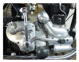
The gearbox outer cover on modern Bullets is prone to flexing when the clutch lever is pulled in, resulting in the loss of clutch lift. The small support kit will help alleviate this flexing by supporting the outer cover from the inside.
