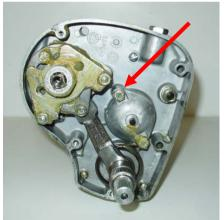
3. . . . so that it looks like this. Remove the bolt (arrowed).
