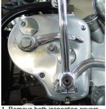
1. Remove both inspection covers, neutral lever, eccentric bush bolt, gear lever, kickstart lever and four cover retaining screws . . .
