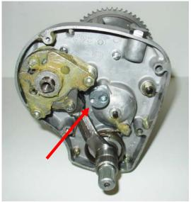
4. Screw the stiffener block into the vacant hole, using the Allen head screw with the coarse thread . . .
