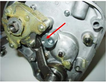
5... until it is roughly in this position (note position of threaded hole). You need to line up the central hole in the outer case with the threaded hole (arrowed). Push the cover back on and looking through the central hole, you should just be able to see the vacant hole in the stiffener block. Adjust the block until the holes line up, then tighten the block securing screw.
