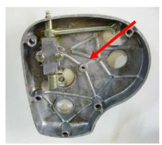
7. When you refit the gearbox cover and depending on the model/year of your bike, you may need to carefully remove a small amount from the top of the central mounting hole casting, until the cover fits flush.
