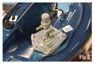
Remove throttle cables, cold start cable, all connections, airbox rubber from the throttle body. Then unbolt the inlet manifold from the cylinder head and remove the throttle body and inlet manifold as one unit from the bike. (Fig 3)
