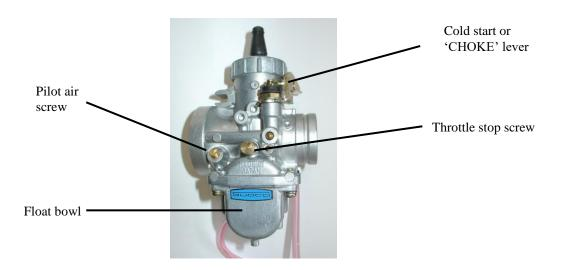
To set correct tickover (or idle) speed, start engine and allow it to its reach normal running temperature. Adjust the throttle stop screw to achieve the slowest possible idle speed. Now adjust the pilot air screw for fastest engine speed. Reduce engine speed with throttle stop screw again, repeat the same series of adjustments once more.
