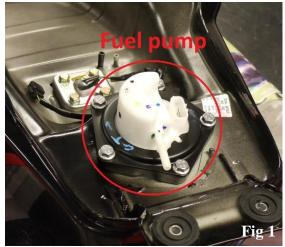
Take the fuel pump adaptor plate and oring and bolt in place of the fuel pump using the original bolts. Take the fuel tap, two Allen key bolts and two copper washers and bolt tap to adaptor plate ensuring the correct orientation. (Fig 2)
