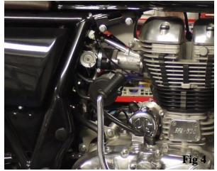
Both the cold start and throttle cables can now be removed from the bike. Fit the new throttle cable supplied in the kit to the throttle end and route suitably ready to fit to the carb. Fit the "rubber bung" in place of the inlet pipe to the airbox. (Fig 5)
