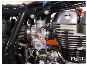
Fit the fuel pipe onto the carb and secure with clip. Fit the tank back in position along with the new breather pipe fitted to the original outlet previously used for the carbon canister (The larger pipe located on the underside of tank). This breather can then be routed down the bike and facing the ground into open air. (Fig 12)
