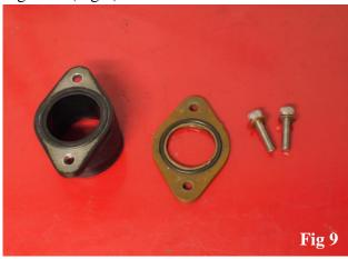
Use this black manifold along with the spacer, two bolts and two o-rings already removed from the bike to bolt back onto the head. Fit the new head steady bracket and longer bolts in place of the oringal setup. (Fig 10)
