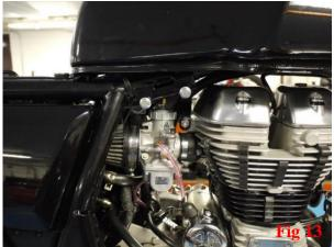
Adjust throttle cable if required and check the throttle returns fully in all positions. Refit seat, battery, covers and test bike. The carb is supplied with a base setting and there are some additional jets included to aid with fine tuning.
