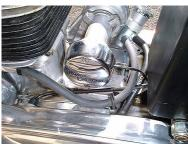
**4,** Screw the assembled sleeves into the threaded hole now left in the crankcase where you have removed the alloy oil filler neck. Tighten as much as possible by hand, ensuring that the inlet and outlet unions are positioned as in the picture on the left (if necessary use a pair of grips on the knurled section).
